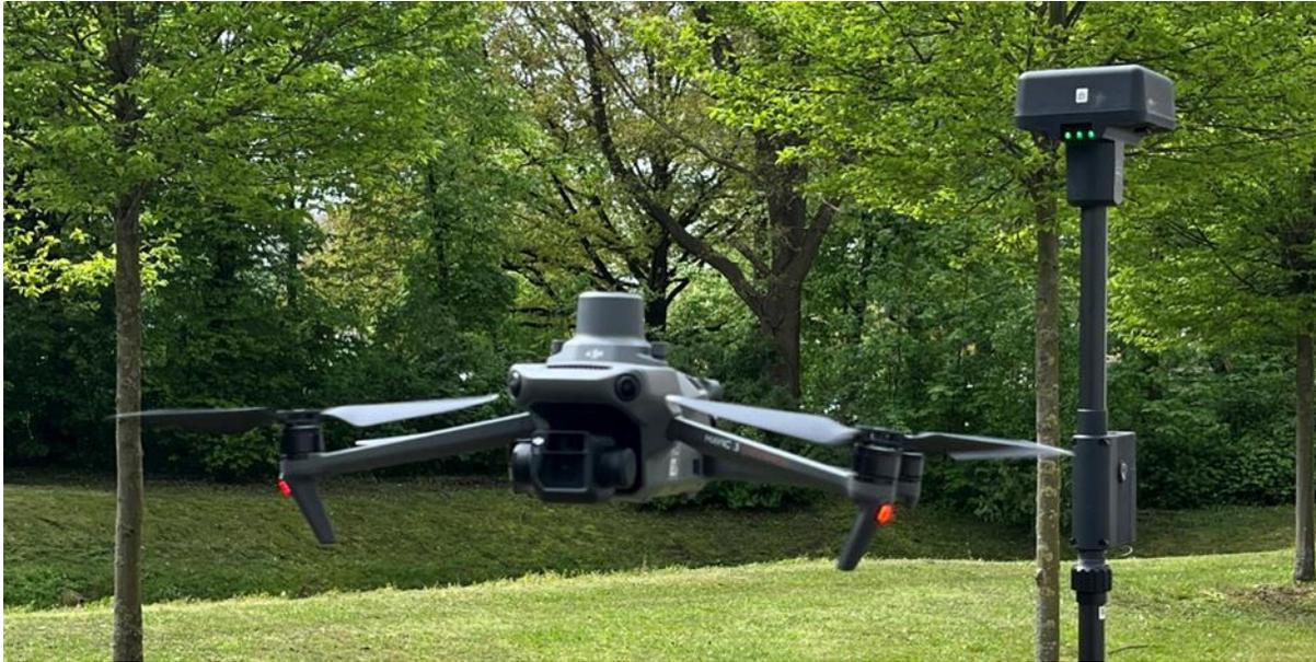
**Figure 5.** DJI Mavic 3E with RTK antenna.
