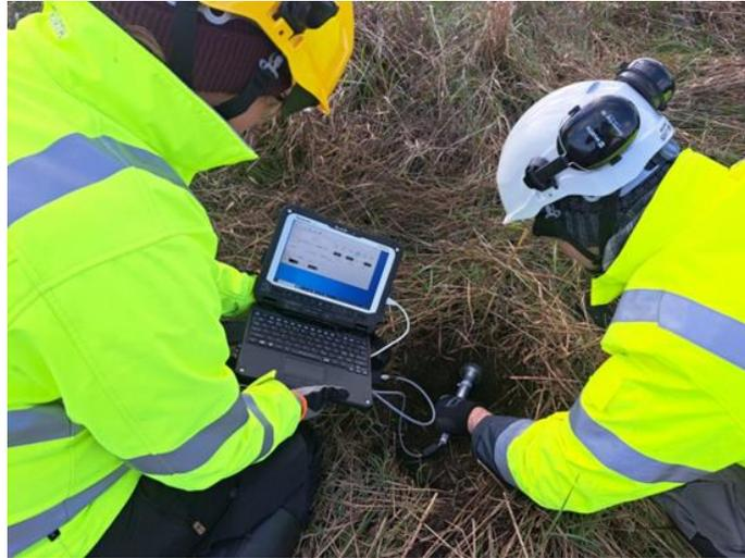
**Figure 1.** Organic soil dielectric constant measurement using hand-held percometer.
