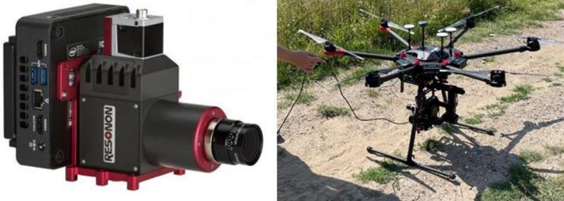
**Figure 11.** Hyperspectral camera Resonon Pika L. (a) Standalone camera; (b) Camera installed on the Ronin MX on DJI Matrice 600 Pro.
