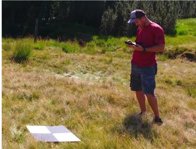
**Figure 13.** GCP's measured by the GNSS technology.
