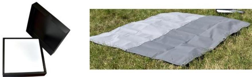
**Figure 12.** Calibration targets; (a) Spectral Evolution Reflectance Target (spectralon); (b) Resonon Calibration Canvas.
